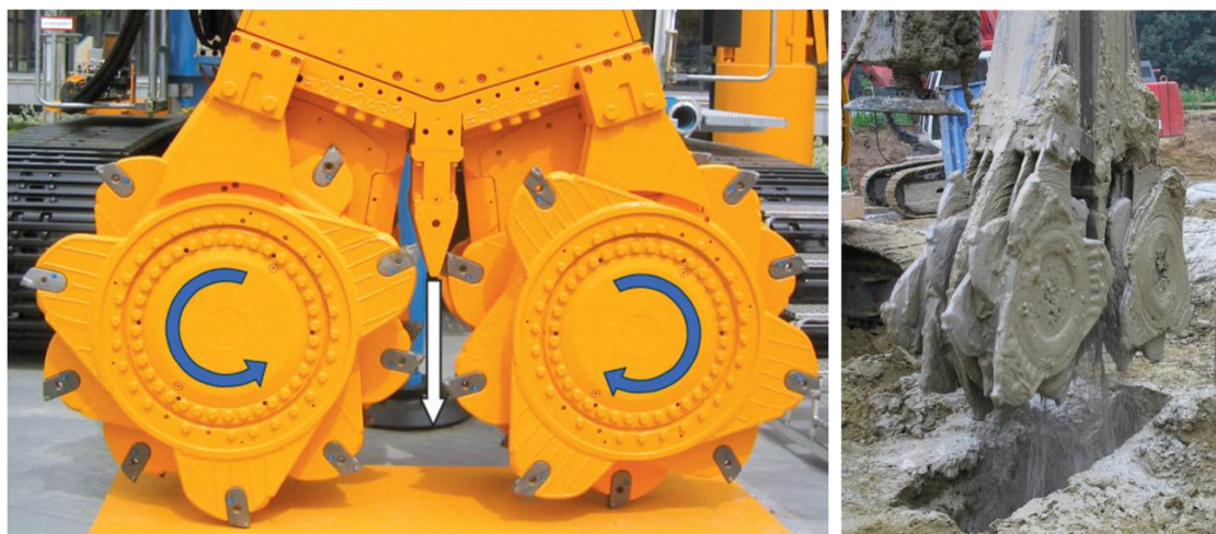
Figure 6: The cutting wheels of the CSM machine
