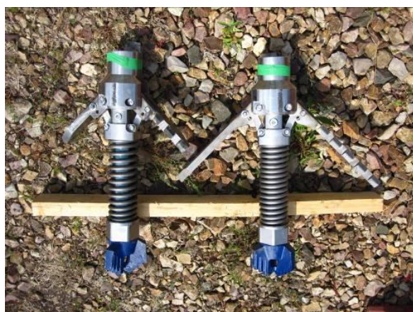
Figure 4: Soletanche Bachy Springsol ® systems with 400 mm (left) and 600 mm (right) diameters, after Guimond-Barrett et al. (2012a)
